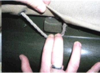
Loop the rope under the tabs on the body panels. Do on both sides of the Land Rover
