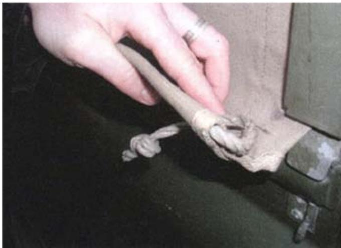
**Tie a knot in the rope on the curtain sides (at the front of the vehicle) to form a loop.**
