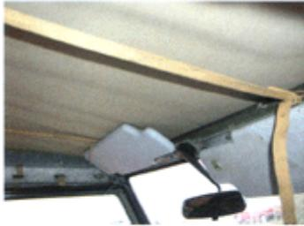
Hook or thread straps at the front on or through the windscreen rail, and tighten up
