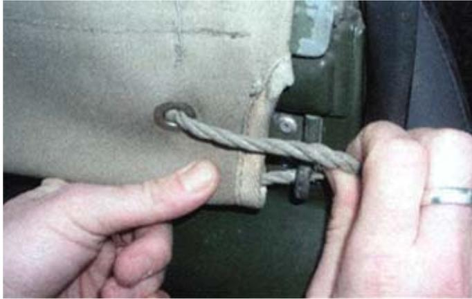
Fit the loop at the front (on both sides) over the fitting by the rear of the door.
