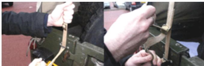
Pass the rear webbing strap down and through the tailgate loop and buckle up
