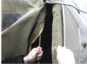
Thread the rope on the tailgate flap through the outside of the eyelet on the curtain sides
