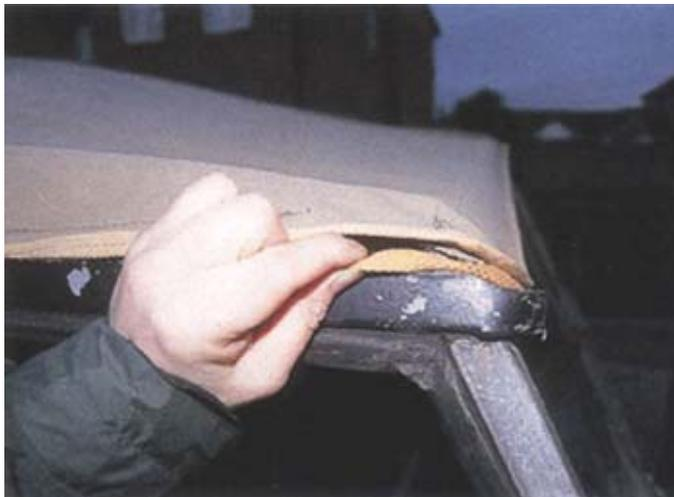
Pull the webbing tight and hook on to the gutter rail tabs above the door.
