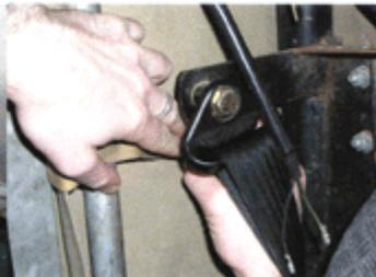
Tighten up the curtain side straps inside (partially obscured by the seatbelt mounts)
