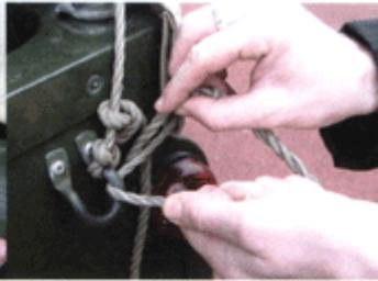
Pull the rope tight on both sides, and tie the end to the hoops on the rear quarter panels
