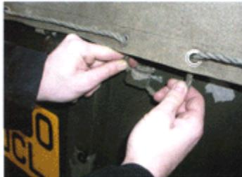
Loop the rope under the three tailgate tabs pulling the rope through after each one...
