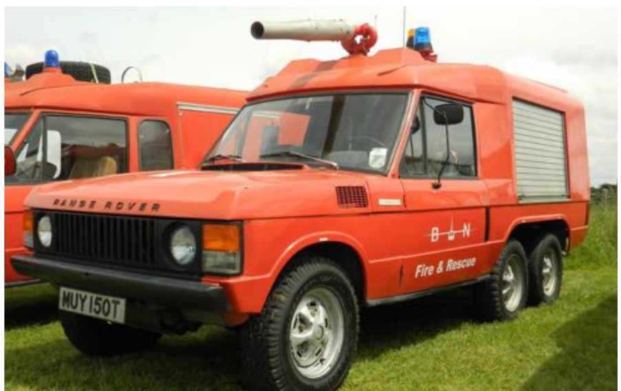
The three-axle Range Rover was much liked as an RIV. This is a 1979 two-door model, with the GRP bodywork typically fitted.
