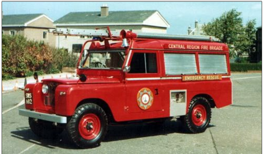
This Series IIA 109 for the Scottish Central Region Fire Brigade had an individual design, but the mid-mounted control panel for the fire pump was typical of Carmichael.
