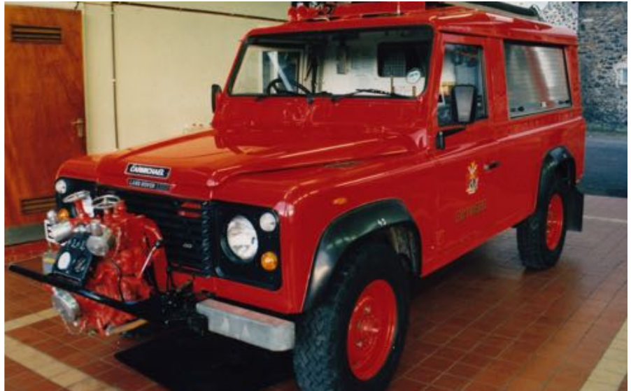
One Tens tended to have front-mounted pumps rather than the traditional Carmichael mid-mounted type. This is a 1987 example.
