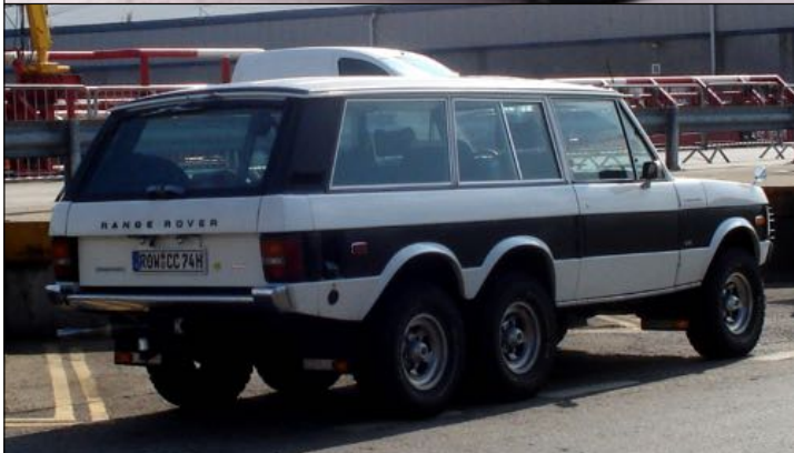
A few Commando chassis were given estate-type bodies. This LHD example is typical. The first one may have been the one that Wolfrace Wheels used to advertise their products in 1976. (Gordon Black photo)
