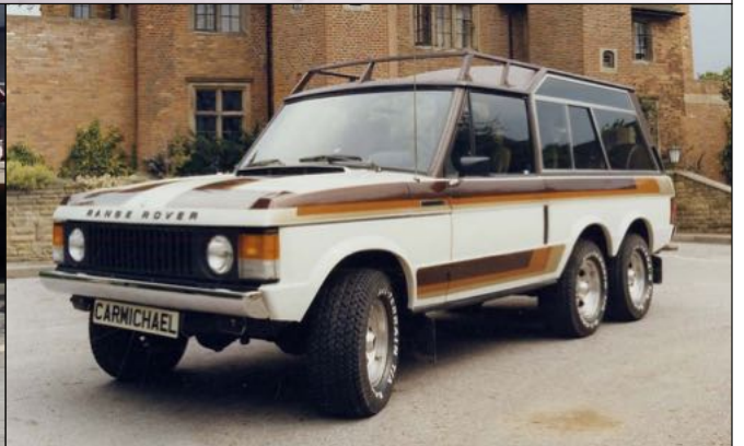
Last photo for now.... The three-axle chassis was exploited further with special bodies by Carmichael Custom Cars. This is the two-door Highlander model.lv
